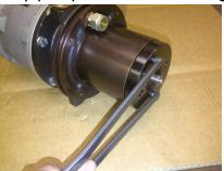
11. Remove and replace inner O-Ring (Item 42) from suction check valve.
