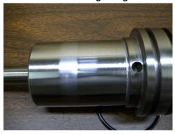
34. Using fingers or Teflon block ONLY, install new Teflon seals in grooves of oil piston. The seals will remain stretched.
