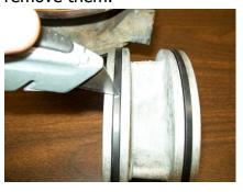
26. Carefully remove O-Rings (Item 100) from air piston. Inspect the air piston for damage.
