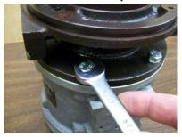
10. Lay pump on its back. Using a spanner wrench, remove suction check valve.
