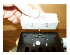
49. Reinstall air valve and tighten.
