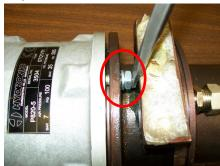
15. Carefully pry between air and oil chambers and then pull air chamber off.
