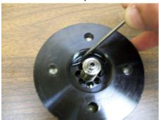
12. Remove and replace outer O-Ring (Item 37) from suction check valve.
