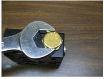
9. Remove all of the 13mm bolts holding the air chamber to oil chamber. There should be 5 total. (Item #26)
