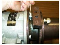
47. Reinstall air manifold with open muffler port pointing at oil chamber and tighten it down. Install the muffler.
