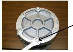
17. Using a wood or plastic hammer handle or something similar, knock off cap (Item 14) of air chamber from inside. Inspect the inside of the air chamber for scratches.
