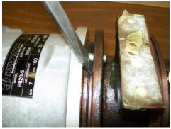
16. Remove the 13mm bolts from top of air chamber. There are 6 total. (Item 13)
