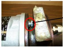
14. Pry on 13mm nut to separate air chamber (Item #19) from oil chamber (Item 25) and remove nut and washer.
