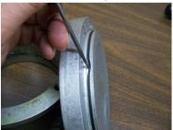
19. Using a 90° angled pick, remove both brass plugs from the air chamber. There is one on each end. (Item 20)
