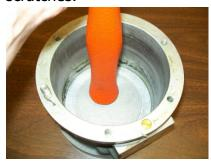
18. Remove and replace O-Ring from air chamber cap. (Item 15)
